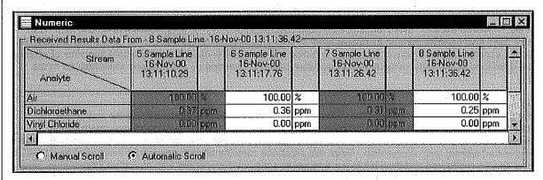
No limits on the number of components are imposed by the software, which can present raw mass spec data, online calculations (derived values) system parameters and external analog signals in addition to the calculated gas concentrations as shown above.
