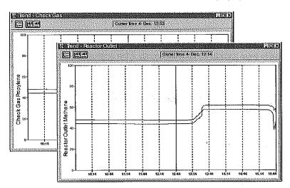
Each new trend form is configured using a set-up wizard which provides easy analyte and stream selection, axis configuration (log mode, linear mode, manual & automatic dynamic range, time, etc.) and trace color. Where a complex set of axes is required to present both logarithmic and linear plots on a single form then multiple y-axes are supported. Each form can be positioned and sized in order to make the best use of the available display area.
